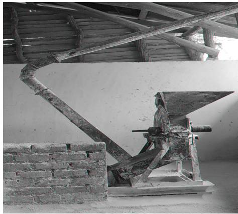
Figure 1: Swing hammer mill being used for lime milling in Malawi. ©Practical Action.
